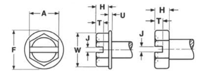
UnSlotted Hex Slotted Hex Steel UnSlotted Hex Washer Slotted Hex Washer Zinc = MH020-----Z1 Zinc = MHS020-----Z1 Zinc = MHW020-----Z1 Zinc = MHWS020-----Z1 Black Oxide = MH020-----BO
